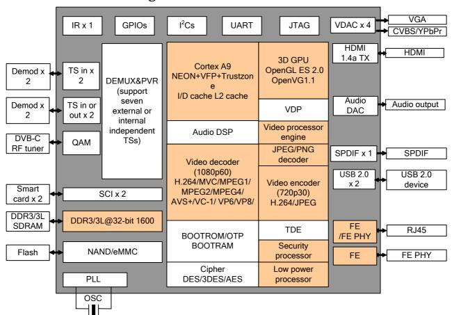
With an integrated ARM Cortex A9 processor and embedded NEON, Hi3716M V400 provides high-speed processing capability that meets differentiated service requirements. It provides a smooth man-machine interface and rich game experience with a
